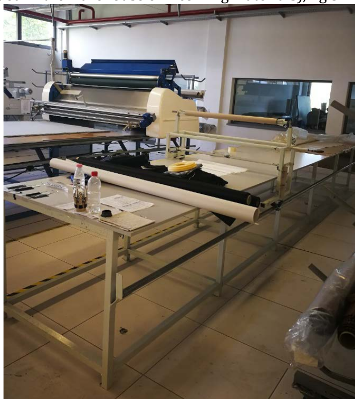
Figure 54. Workplace for manual inspection and spreading of the fabrics/materials
