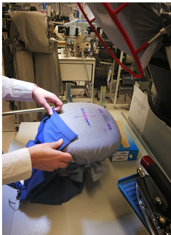
Figure 39. Optimal solution for workplace- bucks for pressing and ironing
