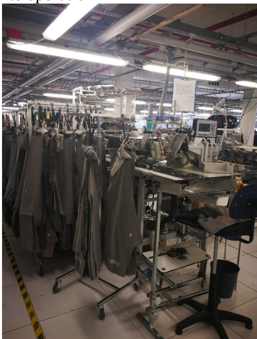
Figure 28. Bundle trucks with clips for the pieces
