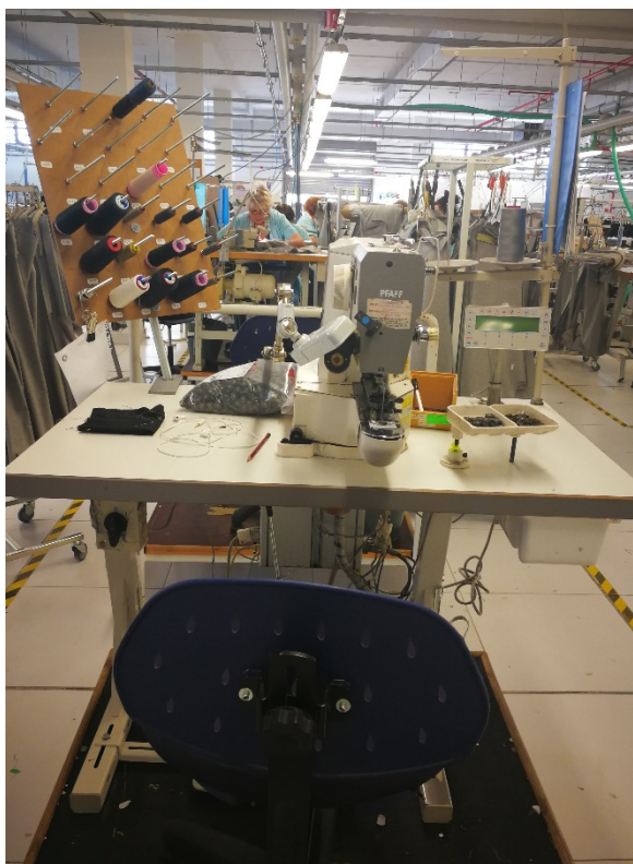
Figure 38. Optimal solution for workplace- button sewing
