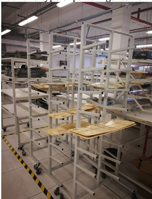
Figure 26. Transport trolleys/shelves for cutted details
