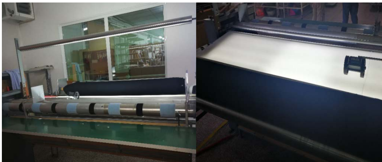
Figure 40. Table for reviewing and measuring input materials
